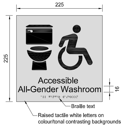
Figure 4.2.7.2: Washroom Tactile Signage
